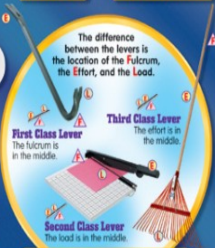
Three Classes of Levers A rigid bar that rotates on a pivot called a fulcrum.
